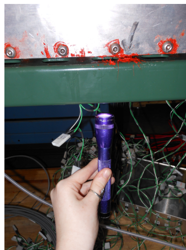
Figure 34: Testing for light leaks
