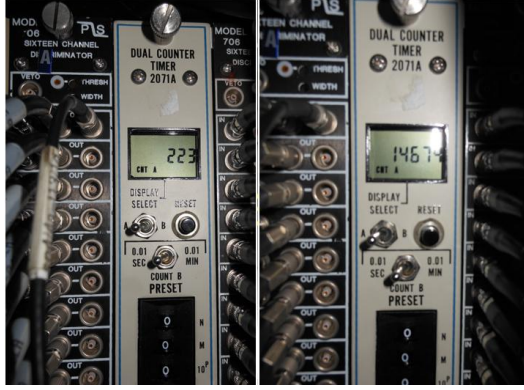
Figure 35: Increase in PMT count rates due to light leak
