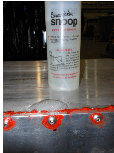
Figure 33: Snoop air leak test
